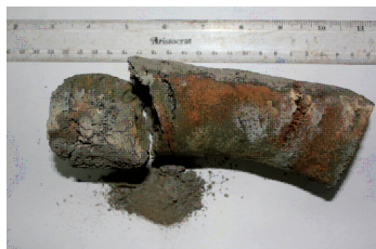
\text{SmCo}_5 alloy prepared by R-D process
