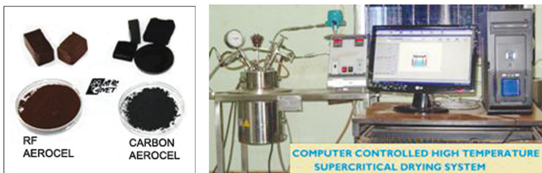
Fig. 1: Photograph of organic aerogel & carbon aerogel (left) & Computer controlled Supercritical Drying system (right)
