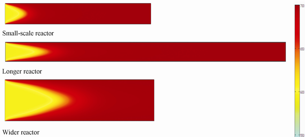
Fig. 2: Temperature field inside the PBMRs (scale in Kelvin)
