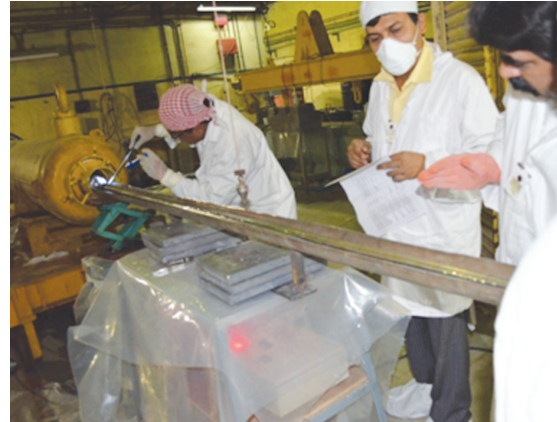
Fig. 4(a): IProMS tool head being inserted inside the pressure tube Q10 at PIED, BARC
